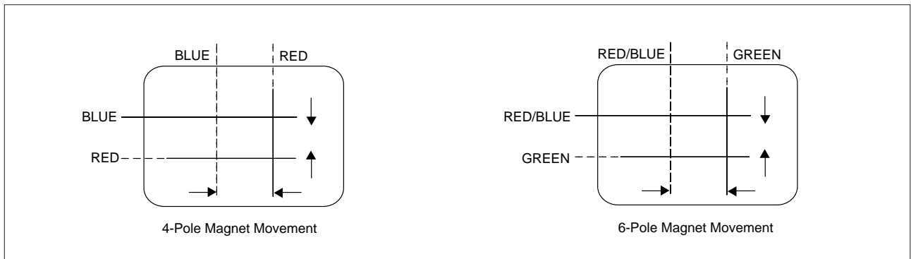
Fig. 4-5 Center Convergence Adjustment
